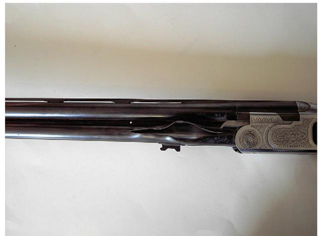
**Figure 2** Example of 12/20 shotgun bursts of the left hand barrel of 12-bore shotguns. The injuries to the left hand and thumb would be highly significant.
